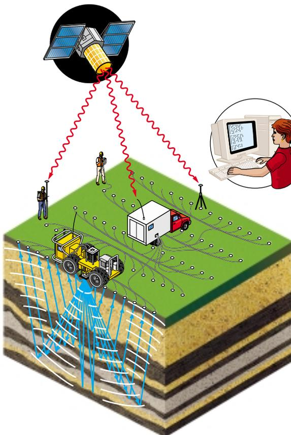
**Figure 5.92** Seismic crews use modern technology to help locate oil and gas. A satellite-based global positioning system identifies the location. Large vibroseis trucks send energy waves into Earth's crust to create seismic waves. The waves are analyzed using computer software.
