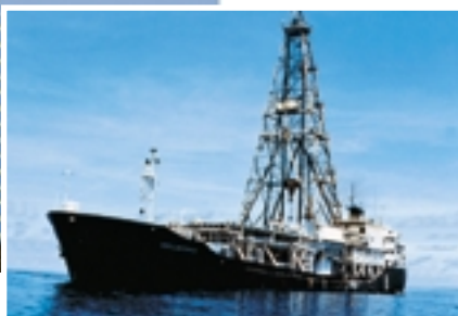
Figure 5.39B The Glomar Challenger used oil-drilling technology to help scientists explore beneath the ocean floor.
