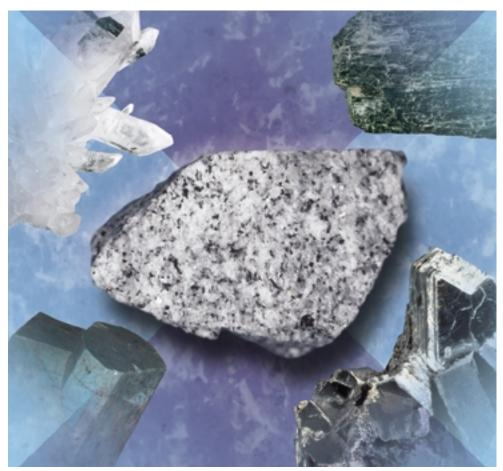
Figure 5.1 Granite is a rock that is made up of an assortment of minerals. It is often polished and used in buildings and at the base of statues. Granite contains the minerals feldspar (sparkling grains), quartz (glassy grains), mica (grey flakes), and hornblende (dark flecks).
