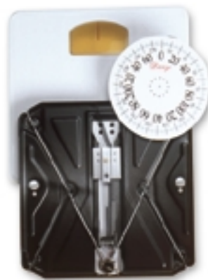
Figure 4.33 A standard bathroom scale is a type of spring scale. Springs within the scale are stretched when a person stands on the scale. The springs are connected to parts that move a numbered scale below a fixed needle.
